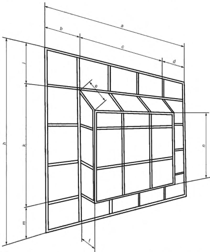
$$S_{\text{КФС}} = a \times j + a \times m + b \times k + \Delta \times k + c \times n + c \times e + c \times f + 2f \times n + (k - n) \times f$$
