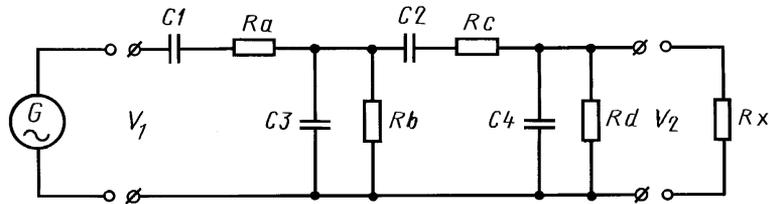
$$(R_a + R_b) \cdot C_1 = (R_c + R_d) \cdot C_2 = 5 \text{ мкс};$$
