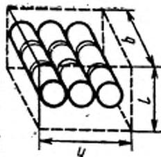
$h \geq 80;$  $l \geq 25;$  $b \geq 40$
